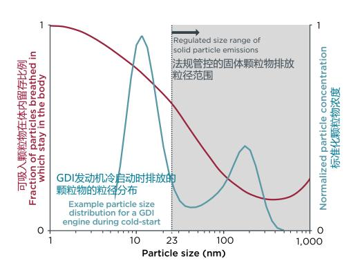
PN is measured as solid particles larger than 23 nm. SPN in the 10-23 nm range are abundant in DI engines, but also in PFI and gas engines.
