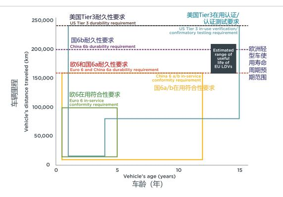
Extending the definition useful life for durability demonstration from the current 160k km for LDVs. **US useful life is 240k km** for LDVs.
